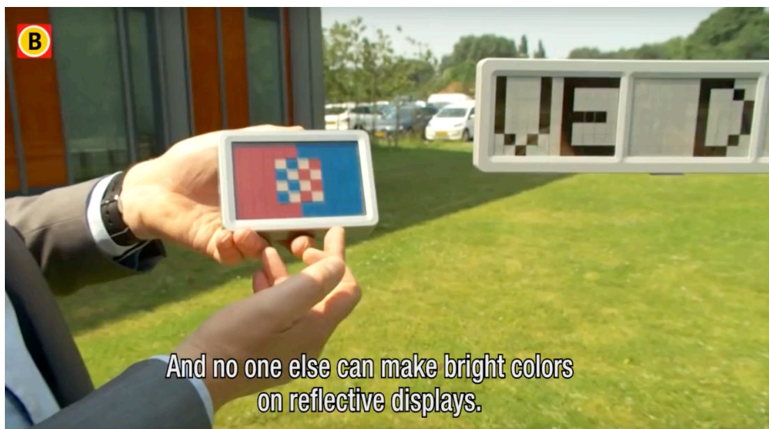
Fig 10. Still [ref 12] demonstrating high contrast in the demo in the top right, and full saturated colors in the demo in the center under extreme sunny weather conditions.
