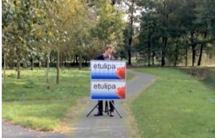
Fig 11: Demonstration of seams in a tiled screen (top) and etulipa's seamless solution using etulipa's patented front optics to hide the seams (bottom).
